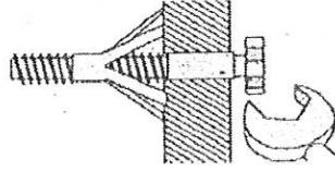
For use when fitting or supporting heavy loads such as shelving, wall cabinets, coat racks.
