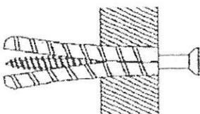
General aerated blocks should not be used to support heavy loads, use a specialist fitting in this case. For light loads, a General Purpose Plug can be used.
